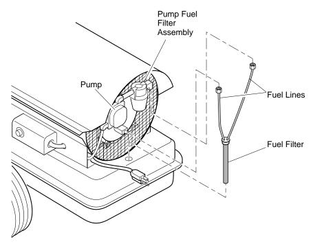
Figure 15 - Removing Tank Fuel Filter
